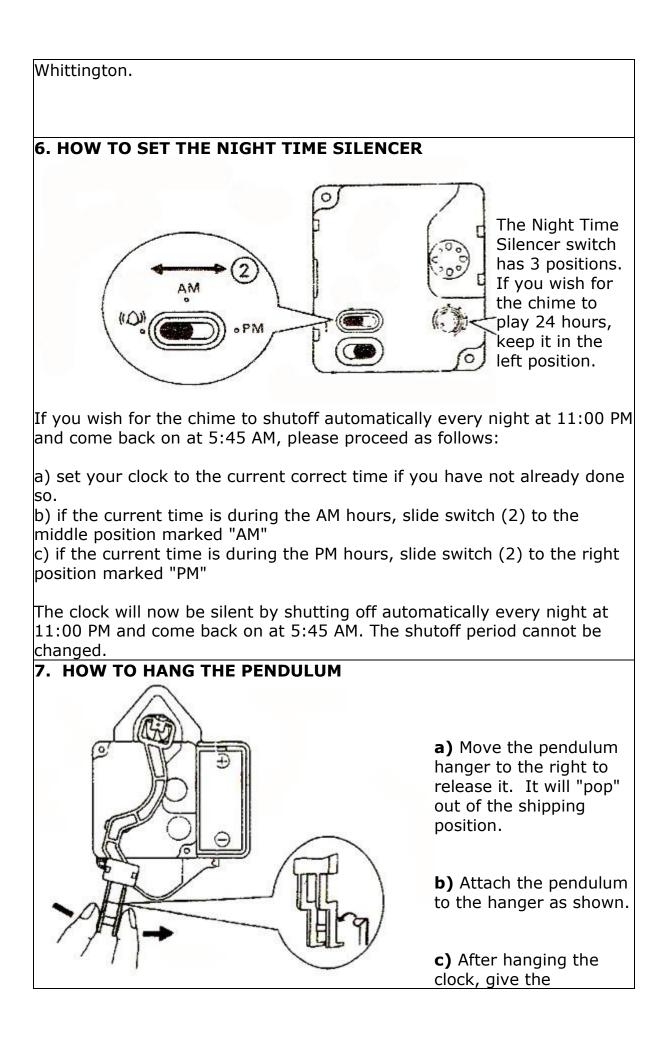
pendulum a gentle push to start it swinging or slightly move the bottom of the case from left to right to start the swinging motion.
